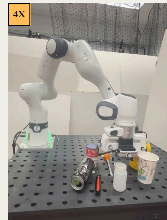
Failed Grasp due to object detection failure !
